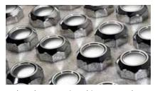
plating processes to endure the temperature changes and weather that a car is subject to outdoors. Triple plating is the most expensive and durable process, which involves plating the steel first with copper and then nickel before the chromium plating is applied.
